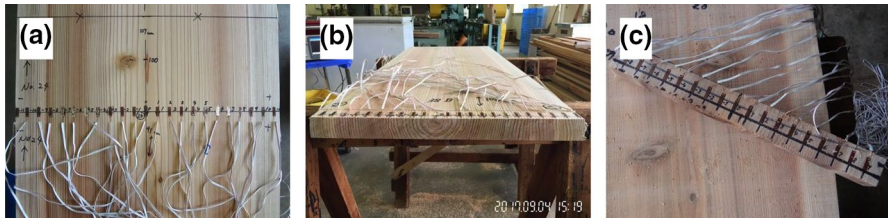
Fig. 4 Measurement of released strain of the residual stress: a strain gauges on a board, b after crosscutting one side adjacent to strain gauges by using a handsaw to release the residual stress, and c a strip after releasing the residual stress
