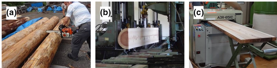
Fig. 1 Log processing: a crosscutting of a 4 m log into 2 m logs, b rough sawing of a board by using a single bandsaw, and c smoothing and thickness tuning by using a planer
