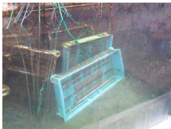
1b 海中暴露試験 1b Under seawater exposure tests
