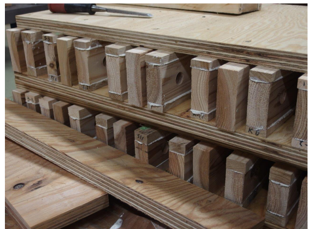
Fig. 2. State of Production of reinforcing nuki of R type
