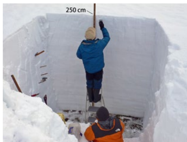
Photo 4. 積雪断面観測 Snow pit observation.
