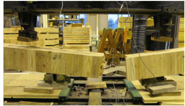
5-layer 7-ply CLT in the minor strength direction (5-7-Mi)
