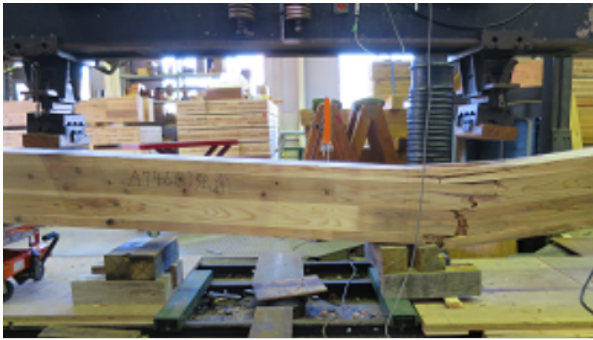
7-layer 7-ply CLT in the major strength direction (7-7-Ma)
