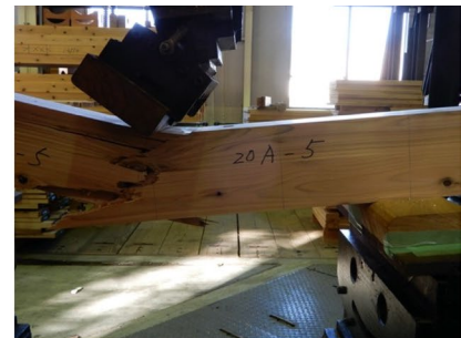
Bending failure in GJ20
