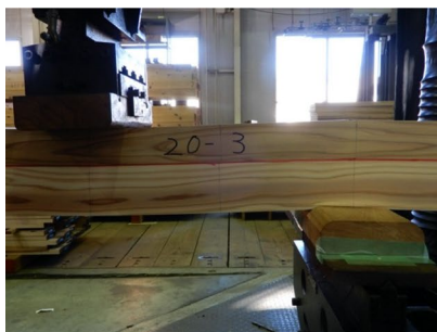
Shear failure at the nonglued edge-joint plane in NJ20
