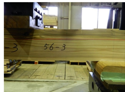
Shear failure at the nonglued edge-joint plane in NJ56
