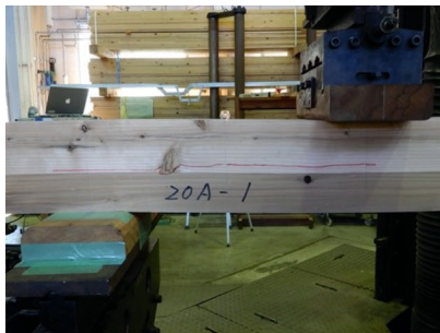
Shear failure near the neutral axis in GJ20
