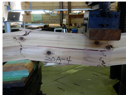
Shear failure at the glued edge-joint plane in GJ20 (bending failure occurred after shear failure)
