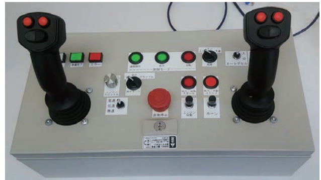
Photo 2. 遠隔操作箱 Remote control box
