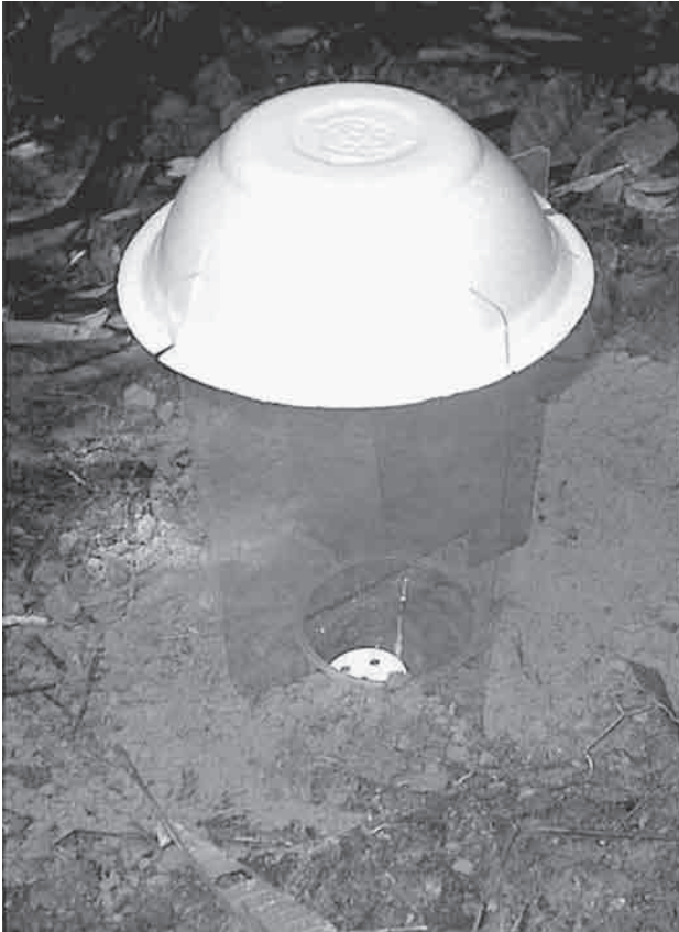
Fig. 2. A flight intercept pitfall trap containing a baited glass bottle with a perforated lid having six holes, each 5 mm in diameter.
