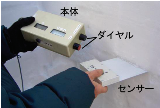
Photo 6. Denoth 式含水率計を用いた含水率の測定 (竹内ら 2009) Measurement of liquid-water content of snow using the snow wetness dielectric device developed by Denoth, A.
