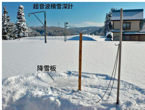
Photo 2. 降雪板 (雪板) と超音波積雪深計 The board for measuring snowfall depth and the ultrasonic snow depth meter
