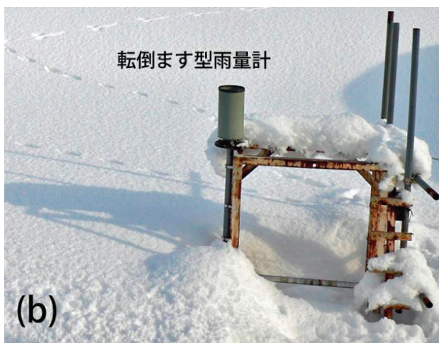
Photo 1. 十日町試験地の気象観測の様子 (a) 気温計 (通風筒) と溢水式降水量計 (風除けとヒーター付) (b) 転倒ます型雨量計 (ヒーター付) Meteorological observations of Tohkamachi Experimental Station, FFPRI (a) Thermometer in the ventilation pipe, and snow and rain gauge with heater and windbreak (b) Tipping bucket rain gauge with heater
