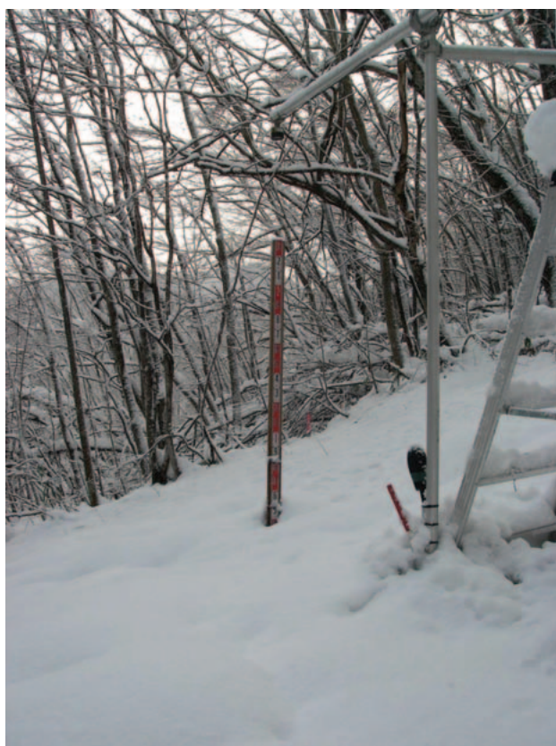
Photo 2. 露場に設置した雪尺と超音波積雪深計 Snow scale and ultrasonic snow depth sensor installed at the meteorological station
