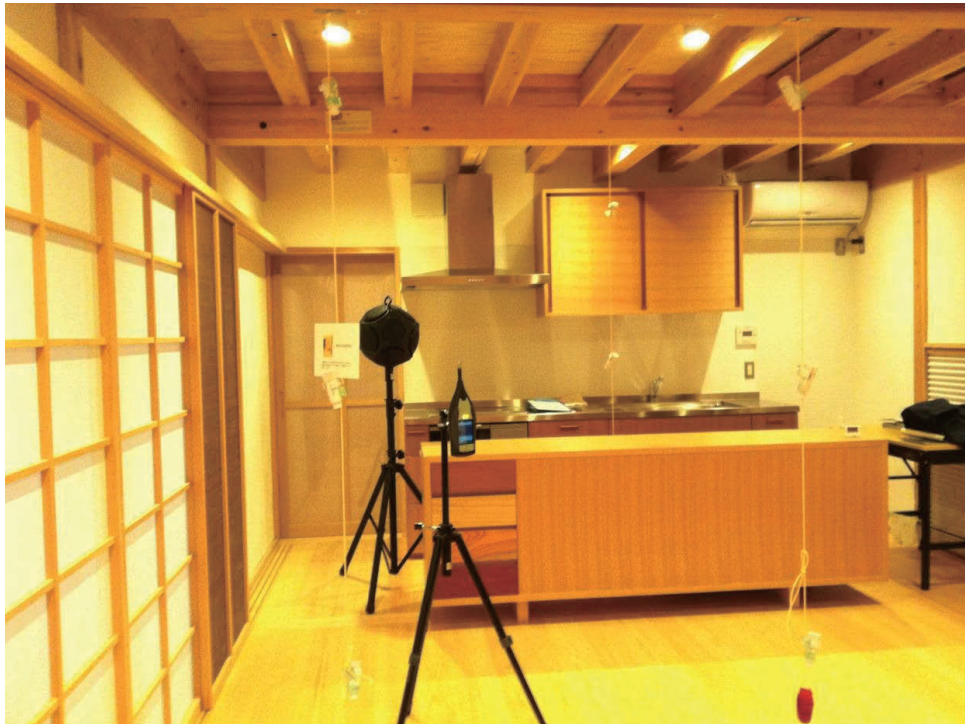
写真 1. 室間音圧レベル差測定のために 1 階の食堂居間に設置された無指向性スピーカーと騒音計 Photo 1. The Omnidirectional speaker and sound level meter which were installed in the dining & living room to measure the sound pressure level difference between the rooms.
