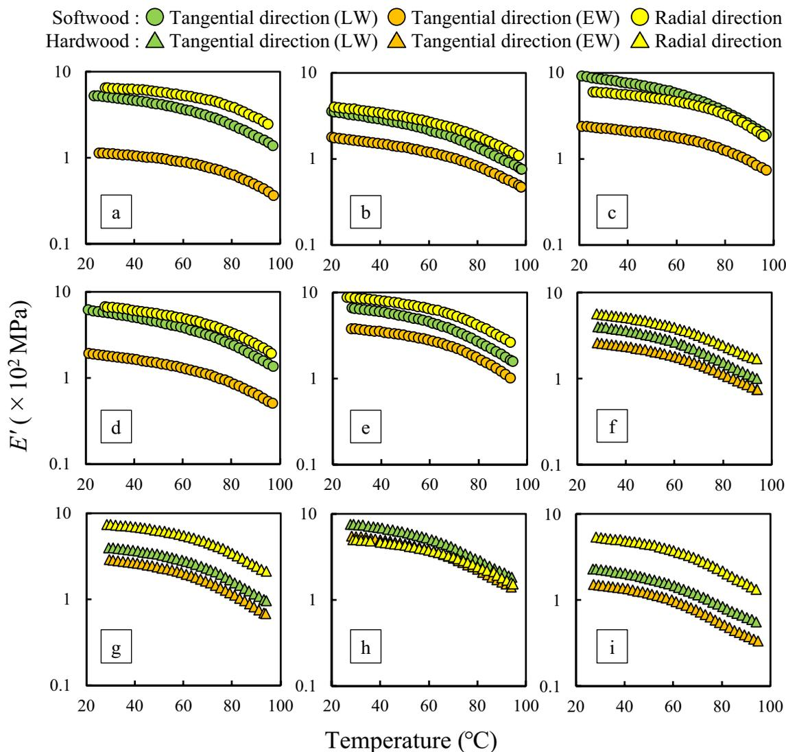
**Fig. 5** Temperature dependence of  $E'$  in tangential and radial direction of some kind of wood swollen by water at 10 Hz. Green filled circles and triangle, LW; orange filled circles and triangle, EW; yellow filled circles and triangle, R specimen. **a–e**, Softwoods. **f–i**, Hardwoods. See Fig. 3 for more details
