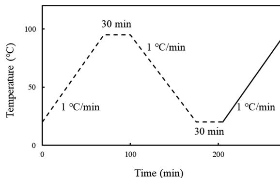
**Fig. 2** Temperature program for measurements of dynamic viscoelastic properties from 20 to 95 °C. Solid line corresponds to the temperature program used in Figs. 3, 4, 5 and 6; dashed line corresponds to the pretreatment process to uniform heating and cooling histories
