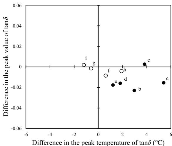
**Fig. 9** Relationships between the difference in the peak value of  $\tan\delta$  and the difference in the peak temperature of  $\tan\delta$  of EW and LW of various wood measured at 0.5 Hz. These differences are EW values minus LW. Filled circles, softwoods; open circles, hardwoods. **a–e**, Softwoods. **f–i**, Hardwoods. See Fig. 3 for more details
