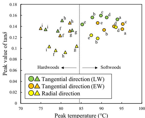
**Fig. 8** Relationships between the peak value of  $\tan\delta$  and the peak temperature of  $\tan\delta$  of EW, LW and R specimen of various wood measured at 0.5 Hz. **a–e**, Softwoods. **f–i**, Hardwoods. See Fig. 3 for more details
