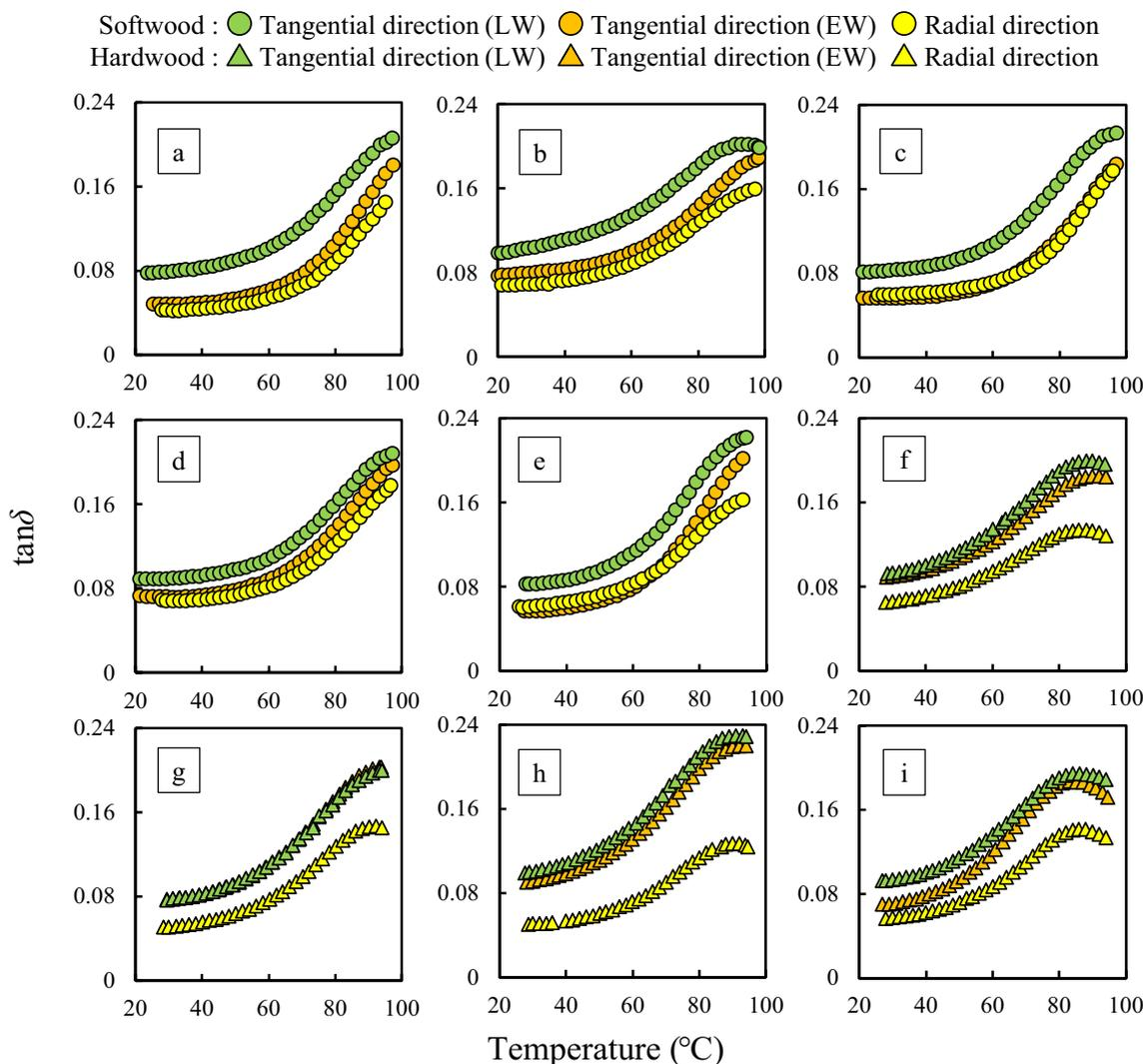
**Fig. 7** Temperature dependence of  $\tan\delta$  in tangential and radial direction of some kind of wood swollen by water at 10 Hz. Green filled circles and triangle, LW; orange filled circles and triangle, EW; yellow filled circles and triangle, R specimen. **a–e**, Softwoods. **f–i**, Hardwoods. See Fig. 3 for more details
