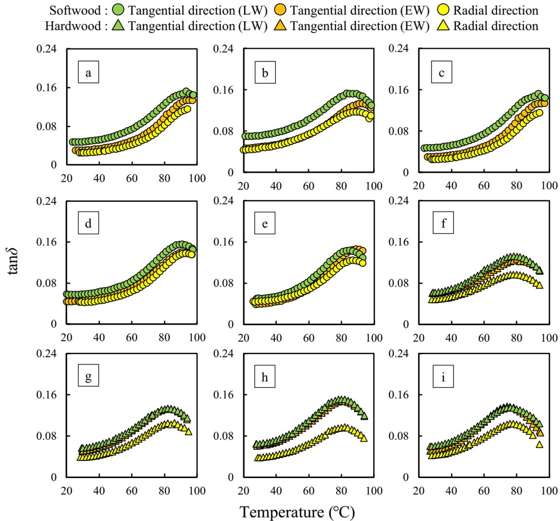
**Fig. 6** Temperature dependence of  $\tan\delta$  in tangential and radial direction of some kind of wood swollen by water at 0.5 Hz. Green filled circles and triangle, LW; orange filled circles and triangle, EW; yellow filled circles and triangle, R specimen. **a–e**, Softwoods. **f–i**, Hardwoods. See Fig. 3 for more details
