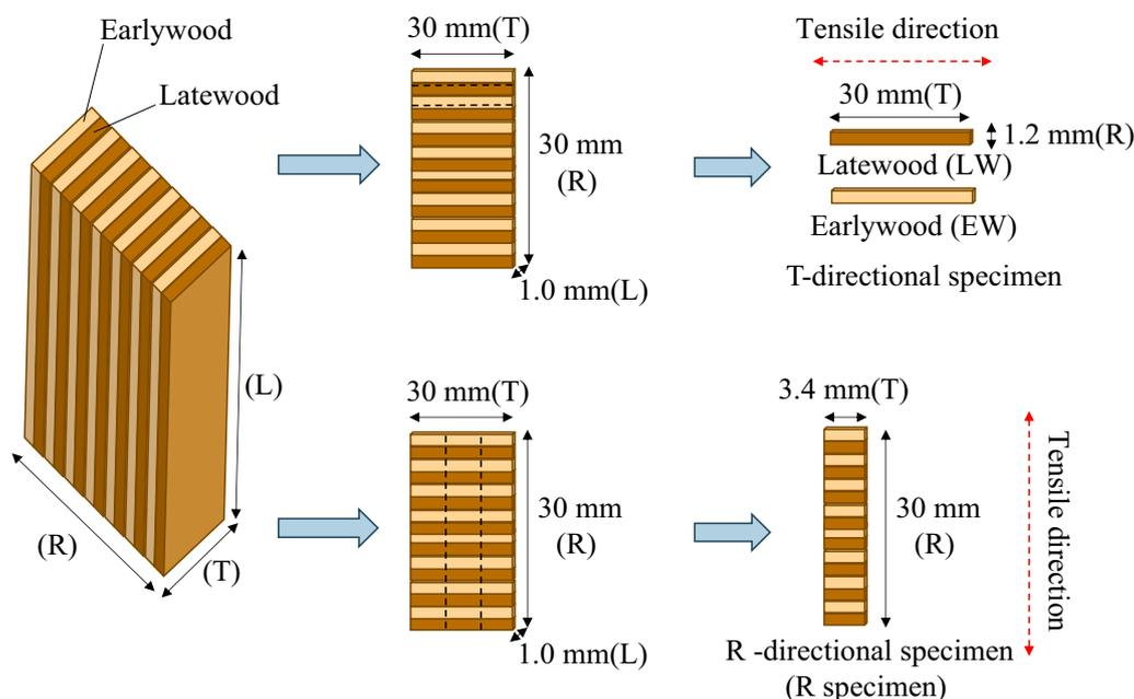
**Fig. 1** Schematic diagram of sample shape of dynamic mechanical analysis (DMA)
