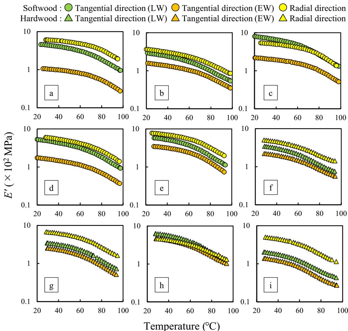
**Fig. 4** Temperature dependence of  $E'$  in tangential and radial direction of some kind of wood swollen by water at 0.5 Hz. Green filled circles and triangle, LW; orange filled circles and triangle, EW; yellow filled circles and triangle, R specimen. **a–e**, Softwoods. **f–i**, Hardwoods. See Fig. 3 for more details
