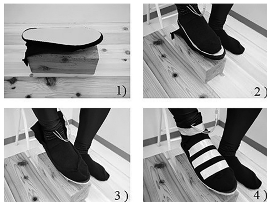
Fig. 1. Attachment of pressure measurement film and foot cover.
